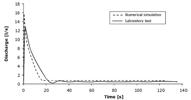
Fig. 4. Comparison between numerical simulation and laboratory test. Air valve diameter equal to 2.0 mm—discharge versus time.
