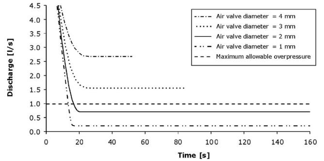
Fig. 1. Discharge versus time: simulation with different air valve diameters and comparison with discharge associated with maximum allowable overpressure
