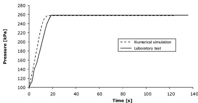
Fig. 3. Comparison between numerical simulation and laboratory test. Air valve diameter equal to 2.0 mm—pressure versus time.
